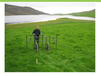
*Figure 15* The Sensys multichannel fluxgate gradiometer system in use at Tingwall (photograph: N. Mehler).
