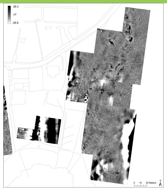
**Figure 21** Shade plot of the enhanced magnetic survey data of areas 7 and 8, overlain on the OS cadastral map (© Crown Copyright/database right 2010. An Ordnance Survey/EDINA supplied service). Grey scale plot clipped at 0.5 standard deviation of the entire dataset (55.0 nT). Map created by J. Coolen and A. Sanmark.
