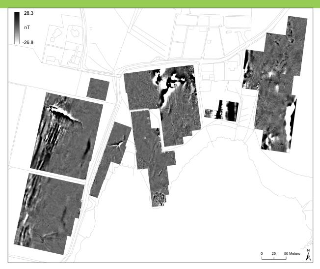
**Figure 16** Shade plot of the enhanced magnetic survey data, clipped at 0.5 standard deviation (55.0 nT), overlain on the OS cadastral map (© Crown Copyright/database right 2010. An Ordnance Survey/ EDINA supplied service). Map created by J. Coolen and A. Sanmark.
