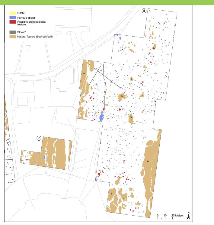
*Figure 22* Interpretation of the magnetic survey in areas 7 and 8, overlain on the OS cadastral map (© Crown Copyright/database right 2010. An Ordnance Survey/EDINA supplied service). Map created by J. Coolen and A. Sanmark.
